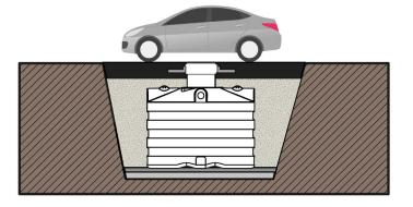
2-6mm washed gravel or Cement-stabilized sand (mixture of concrete sand and about 10% to 15% of cement)
